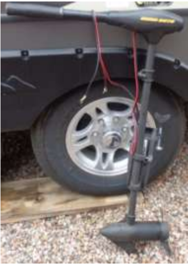
TROLLING MOTOR: Minnkota 5 speed w/Marine Deep Cycle Battery, 30 lb. thrust
